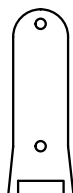
6519 Fail Open Linkage. These have an approximate length of 2.5" and do not have the extra hole for the key override option.
