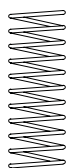
6010 Fail Lock Solenoid Spring. These look the same as the fail open, but are actually lighter in force. Wire diameter is .032". This spring was also used on the 6100 Series Control Head.
