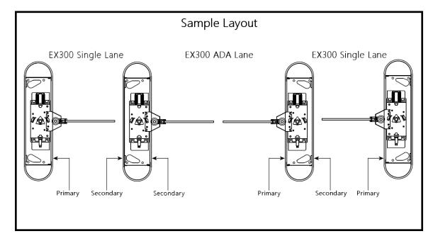
The base ADA lane's secondary cabinet communicates with the primary cabinet with a provided 12 conductor cable. This allows the primary cabinet to operate the solenoids and motor of the secondary cabinet, as well as keep track of the secondary cabinet's arm position via its 3 proximity sensors.
